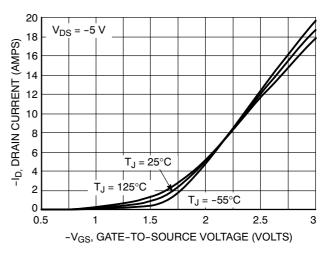
Figure 2. Transfer Characteristics
