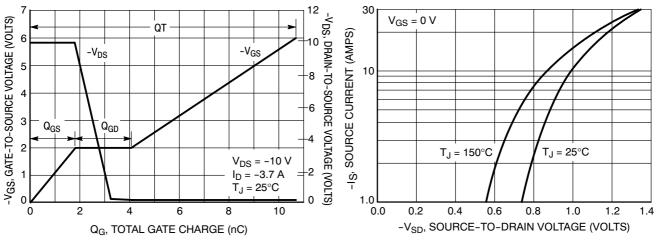
Figure 7. Gate-to-Source and Drain-to-Source Voltage vs. Total Charge
