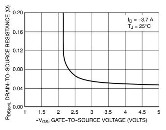
Figure 3. On-Resistance vs. Gate-to-Source Voltage
