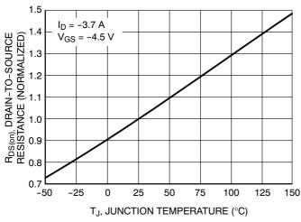
Figure 5. On-Resistance Variation with Temperature
