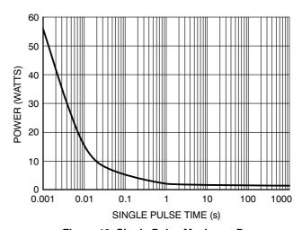
Figure 10. Single Pulse Maximum Power Dissipation
