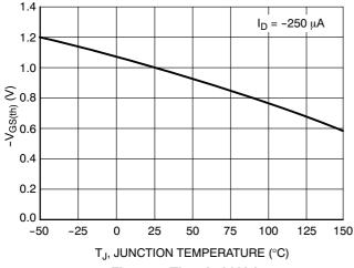
Figure 9. Threshold Voltage
