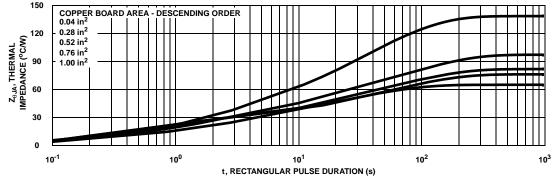
Figure 22. Thermal Impedance vs Mounting Pad Area
