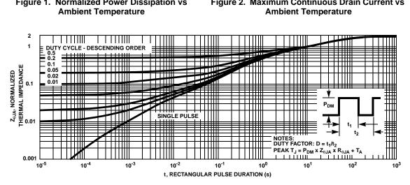
Figure 3. Normalized Maximum Transient Thermal Impedance
