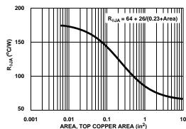
Figure 21. Thermal Resistance vs Mounting Pad Area
