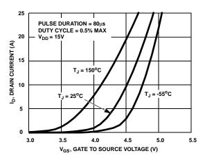
Figure 7. Transfer Characteristics
