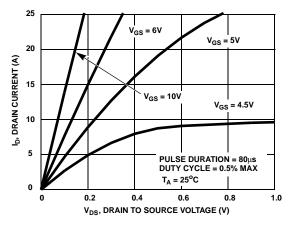
Figure 8. Saturation Characteristics
