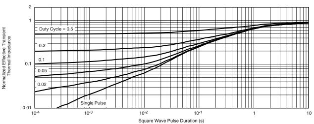
Normalized Thermal Transient Impedance, Junction-to-Foot
