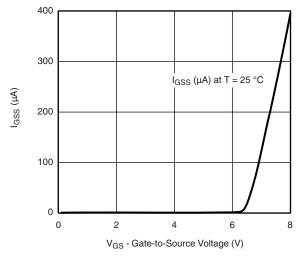
Gate-Current vs. Gate-to-Source Voltage
