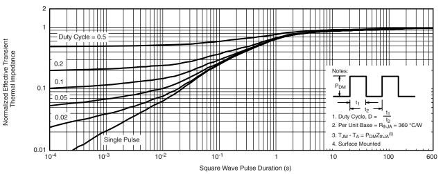
Normalized Thermal Transient Impedance, Junction-to-Ambient
