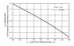
Figure 6. Gate Threshold Variation with Temperature.
