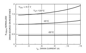
Figure 4. On-Resistance Variation with Drain Current and Temperature.
