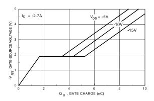
Figure 10. Gate Charge Characteristics.
