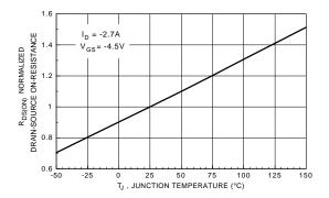
Figure 3. On-Resistance Variation with Temperature.
