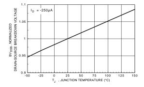
Figure 7. Breakdown Voltage Variation with Temperature.
