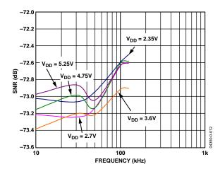
Figure 13. AD7921 SNR vs. Input Frequency at 250 kSPS
