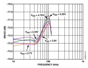
Figure 12. AD7921 SINAD vs. Input Frequency at 250 kSPS
