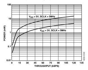
Figure 29. Power Consumption vs. Throughput Rate
