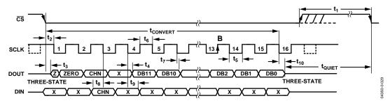
Figure 30. AD7921 Serial Interface Timing Diagram
