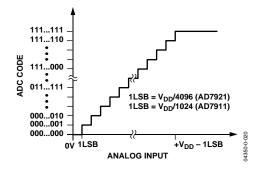
Figure 21. AD7911/AD7921 Transfer Characteristic
