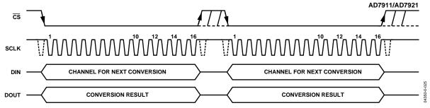
Figure 26. Normal Mode Operation
