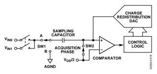
Figure 19. ADC Acquisition Phase
