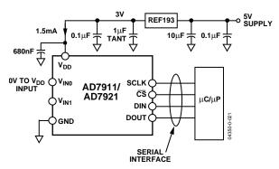
Figure 22. REF193 as Power Supply to AD7911/AD7921
