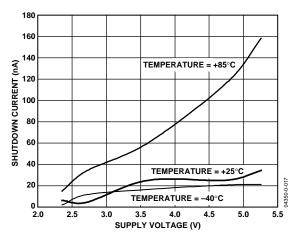
Figure 18. Shutdown Current vs. Supply Voltage
