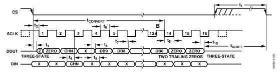
Figure 31. AD7911 Serial Interface Timing Diagram
