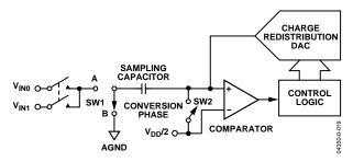
Figure 20. ADC Conversion Phase
