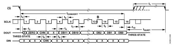
Figure 6. AD7921 Serial Interface Timing Diagram
