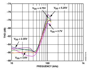
Figure 17. THD vs. Analog Input Frequency for Various Supply Voltages
