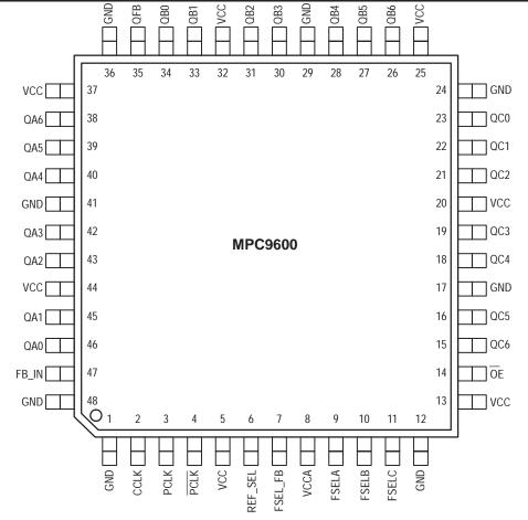
Figure 2. 48 Lead Package Pinout (Top View)
