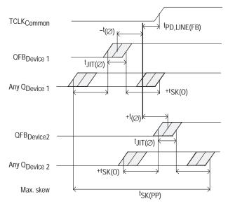
Figure 6. MPC9600 max. device-to-device skew
