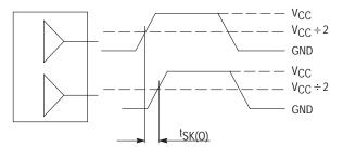
The pin-to-pin skew is defined as the worst case difference in propagation delay between any similar delay path within a single device
