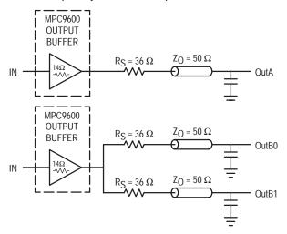
Figure 8. Single versus Dual Transmission Lines
