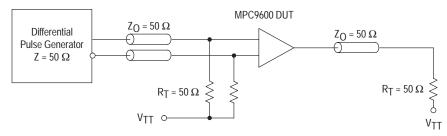
Figure 12. PCLK MPC9600 AC test reference
