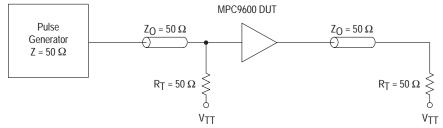
Figure 11. CCLK MPC9600 AC test reference
