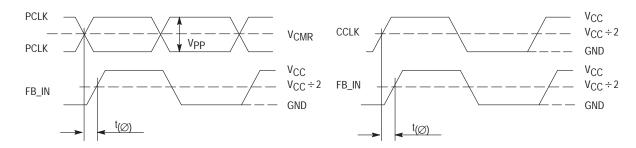
Figure 13. Propagation delay  $t_{(\emptyset)}$ , static phase offset) test reference
