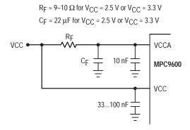
Figure 5. V<sub>CCA</sub> Power Supply Filter
