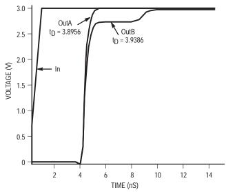
Figure 9. Single versus Dual Waveforms
